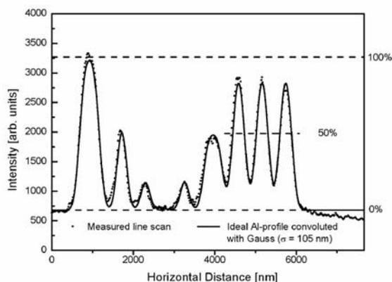
Fig. 5: Comparison of the measured ESCA Al 2p line scan of BAM-L002 with a simulation (convolution of the stripe patterns of BAM-L002 with a Gaussian Point Spread Function of  $\sigma = 105$  nm)
